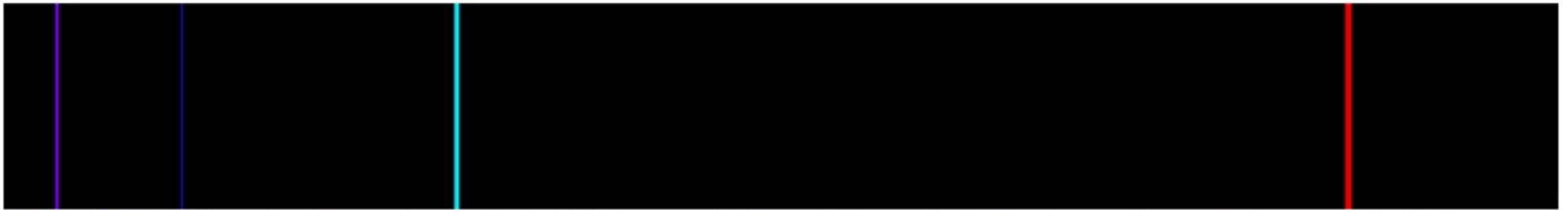
Figure 6.15 The emission spectrum of atomic hydrogen: The spectral positions of emission lines are characteristic for hydrogen atoms. (credit: “Merikanto”/Wikimedia Commons)
